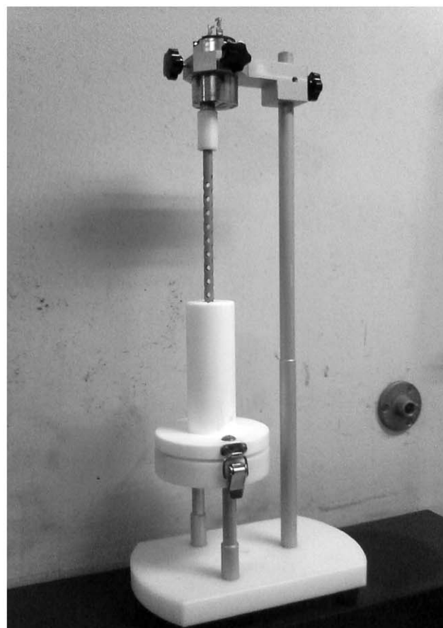
Fig. 2. (A) Simple drawing of plating equipment. (B) Photo of electric plating unit for gold foil target.
